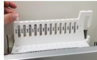
7. Load: Filter Tips, Extraction rack, and PCR rack
