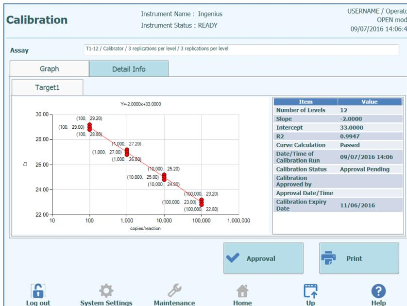
Figure 5-112: Schermata Calibration – Curva standard e replicati
