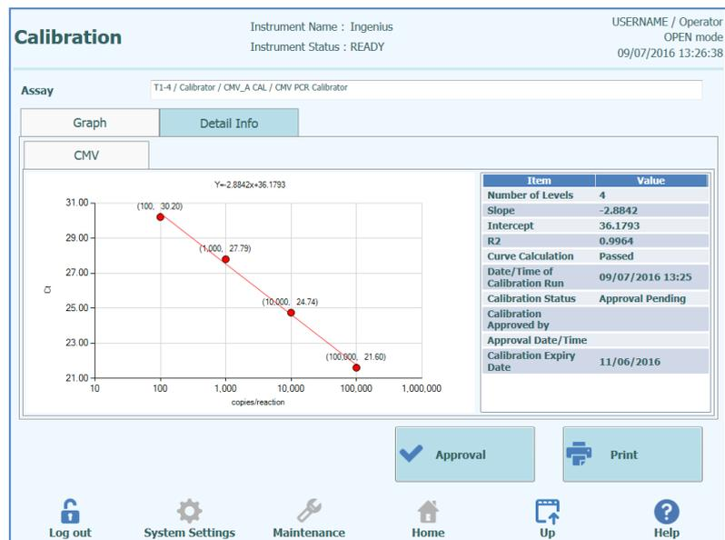
Figura 5-110: Schermata Calibration – Curva standard
