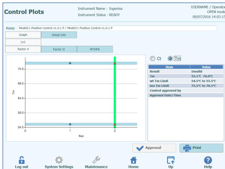
Figure 5-118: Schermata Control – Melting Control Plot
