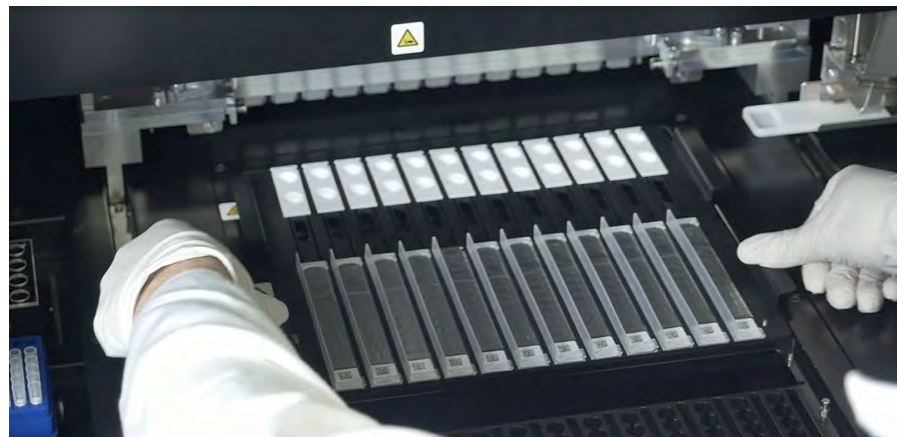
Figure 5-63: Loading Extraction cassette rack on the instrument.
