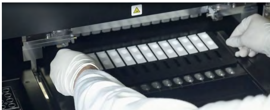
Figure 5-61: Loading PCR cassette rack on the instrument
