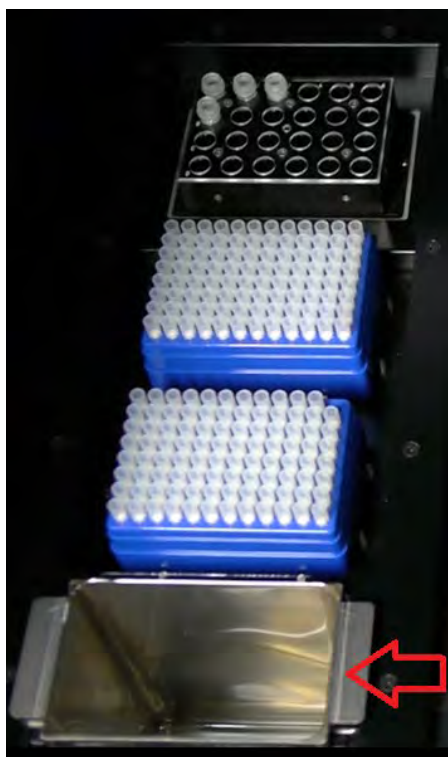
Figure 5-41: Waste container placement on the Instrument.
