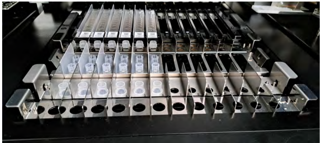
Figure 5-76: Example of Extraction Tube placement in the Extraction Tube Rack.
