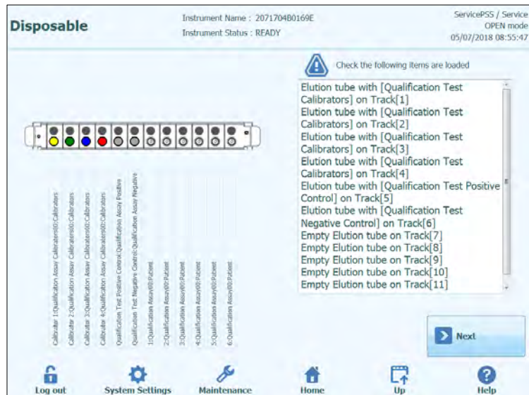
Figure 5-68: Elution Tube (position 1) loading guidance.
