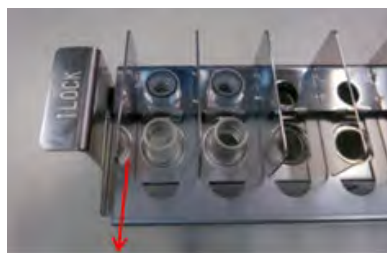
Releasing Sonication Tube Lock from Rack
