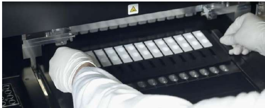
Figure 5-61: Loading PCR cassette rack on the instrument
