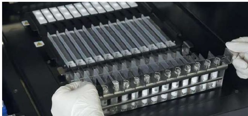
Figure 5-78: Example of Primary Tube loading on the instrument.
