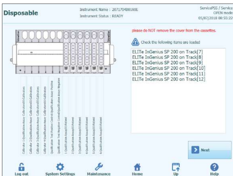
Figure 5-62: Extraction cassette loading guidance.
