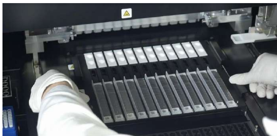
Figure 5-63: Loading Extraction cassette rack on the instrument.
