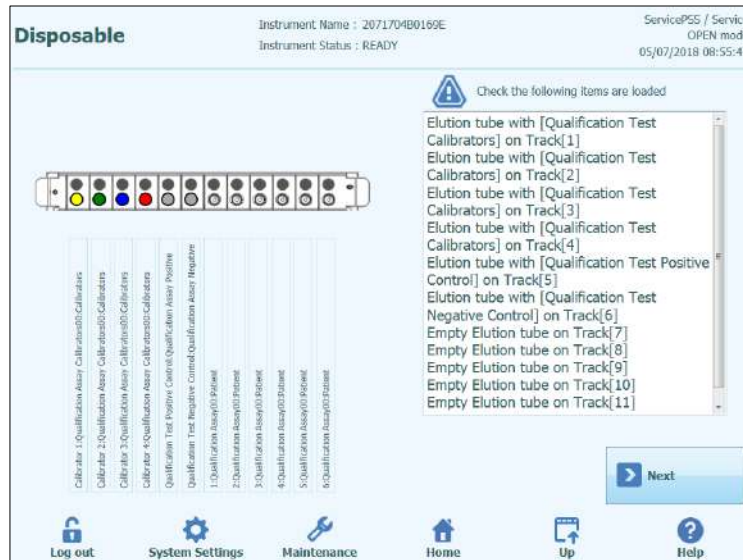
Figure 5-68: Elution Tube (position 1) loading guidance.
