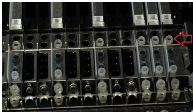
Figure 5-69: Loading Elution Tube Rack on the instrument. Elution tubes are placed in position 1, which is the closest to the front of the instrument
