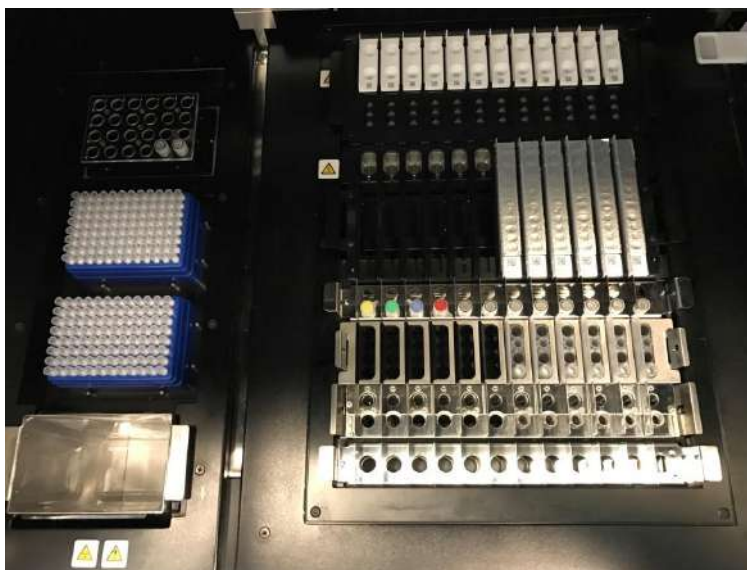
Figure 5-79: Example of final instrument configuration. In this picture it is represented a run configuration that includes: 5 primary samples, 5 extraction cassettes, 12 amplification cassettes.
