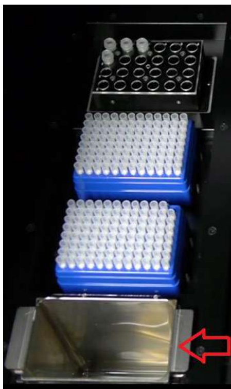
Figure 5-41: Waste container placement on the Instrument.
