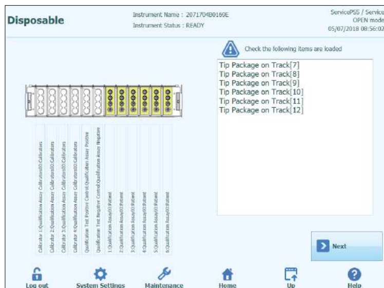
Figure 5-70: Tip loading guidance.
