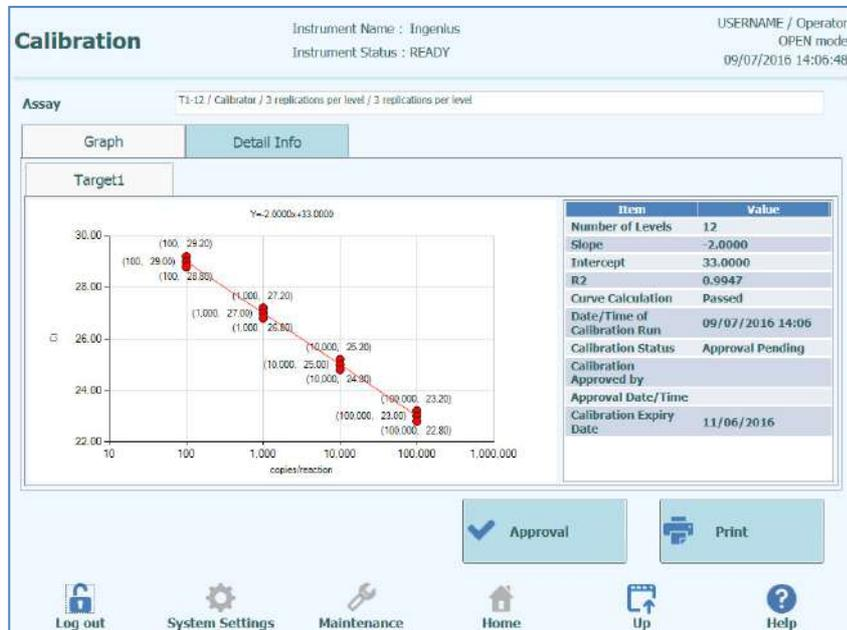
Figure 5-97: Schermata Calibration – Curva standard e replicati
