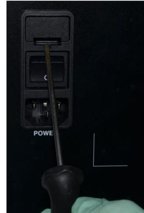
**Fig. 33** Replacing a power fuse
