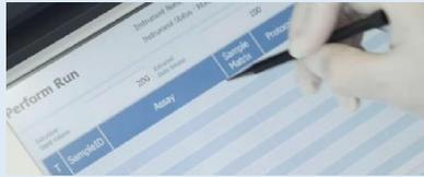
3. Scan the sample barcodes with hand-held barcode reader or type the sample ID
