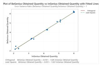
In this test, the orthogonal regression analysis generated a slope equal to 1.026 (95% CI: 0.980; 1.072) and an intercept equal 0.018 (95% CI: - 0.183; 0.219). The linear regression analysis generated a R2 of 0.993.
