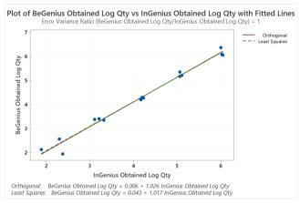
In this test, the orthogonal regression analysis generated a slope equal to 1.026 (95% CI: 0.953; 1.099) and an intercept equal to 0.006 (95% CI: - 0.312; 0.324). The linear regression analysis generated a R2 of 0.983.
