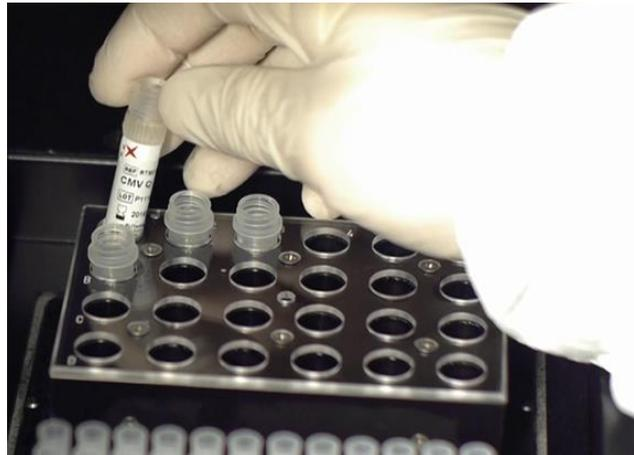
Figure 5-36: Loading / Unloading Inventory on the Instrument.
