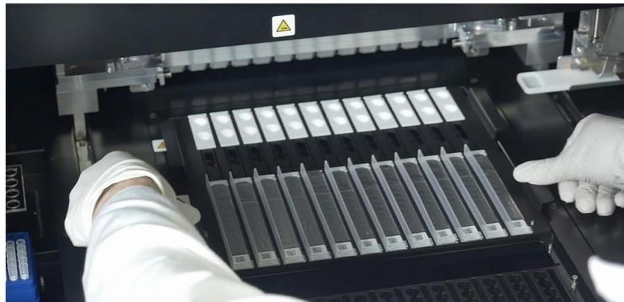
Figure 5-56 : Loading Extraction cassette rack on the instrument.
