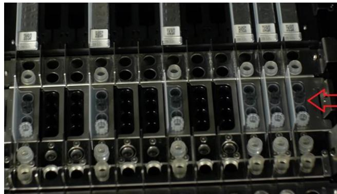
Figure 5-60: Loading Tips on the instrument
