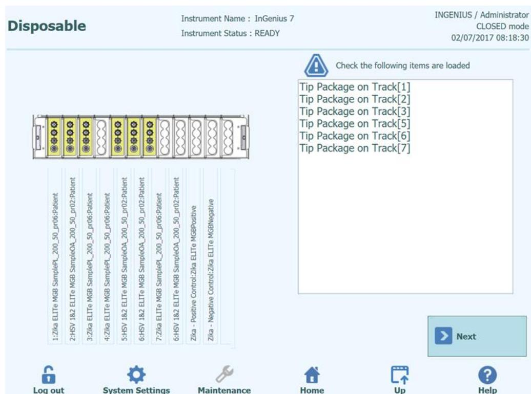
Figure 5-59: Tip loading guidance.
