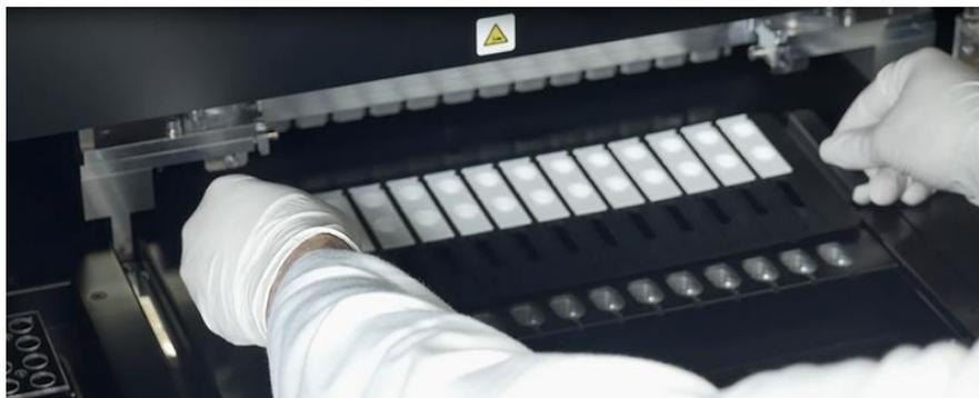
Figure 5-54 : Loading PCR cassette rack on the instrument
