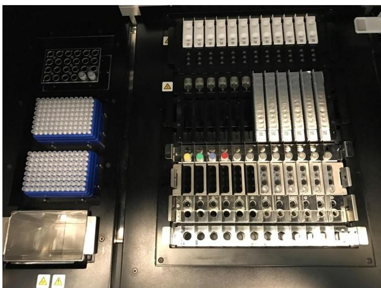
Figure 5-66: Example of final instrument configuration. In this picture it is represented a run configuration that includes: 5 primary samples, 5 extraction cassettes, 12 amplification cassettes.
