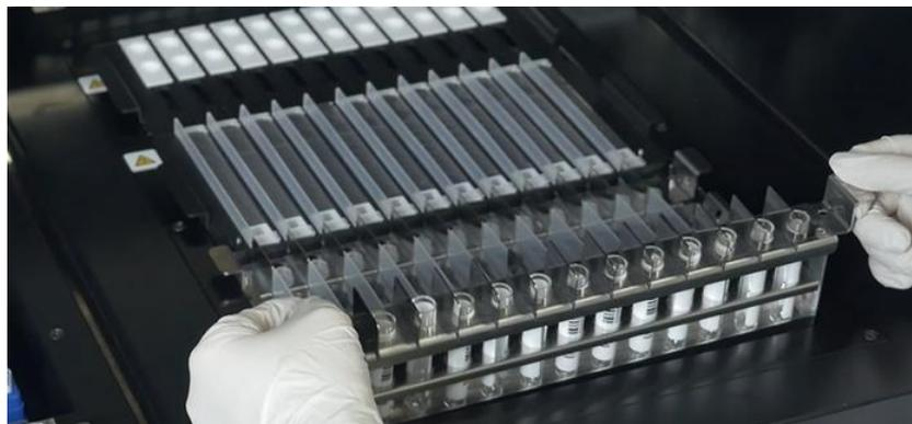
Figure 5-65: Example of Primary Tube loading on the instrument.
