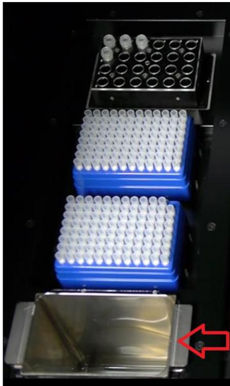
Figure 5-34: Waste container placement on the Instrument.
