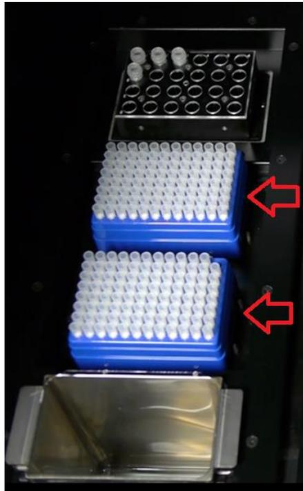
Figure 5-50: Inventory Manager Single Tips placement on the Instrument.
