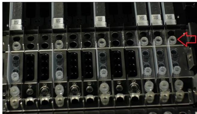
Figure 5-58: Loading Elution Tube Rack on the instrument. Elution tubes are placed in position 1, which is the closest to the front of the instrument
