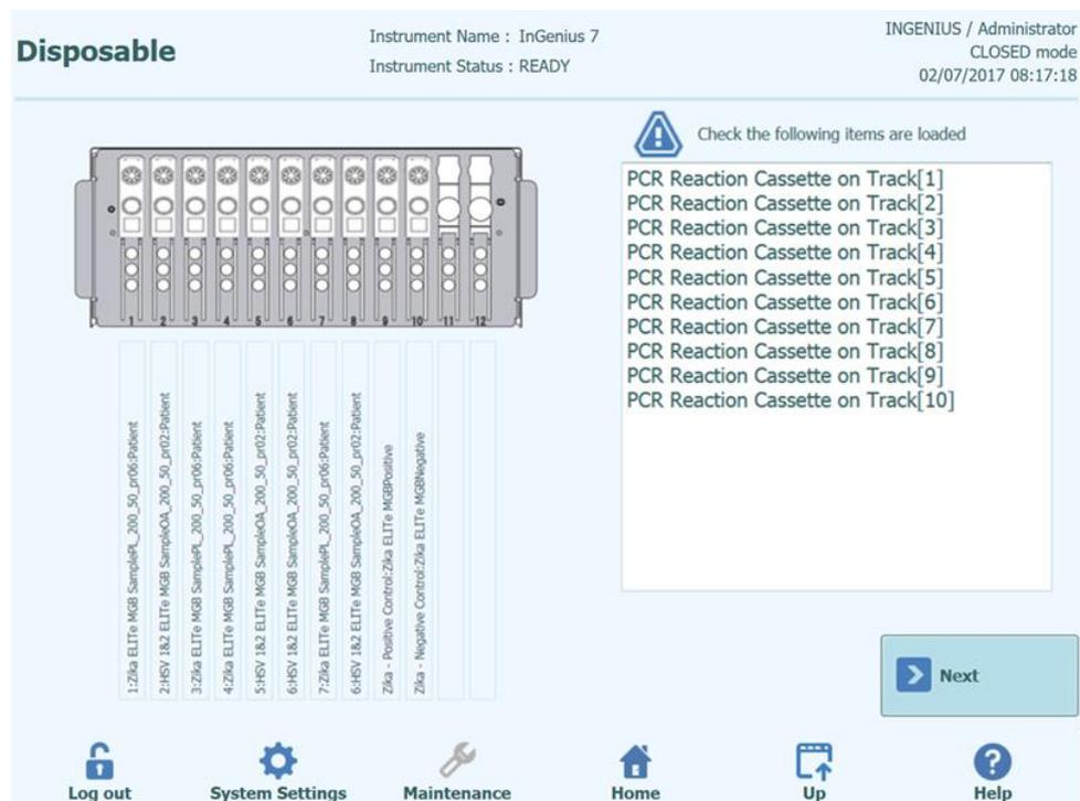
Figure 5-53 : PCR cassette loading guidance.
