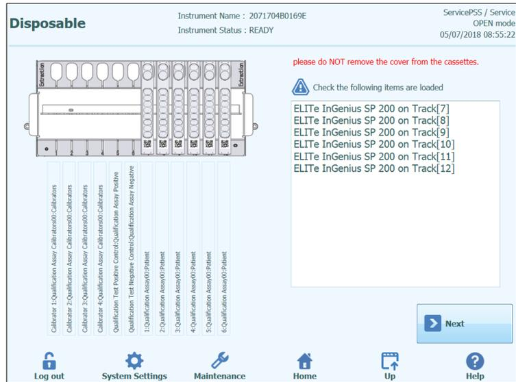
Figure 5-55 : Extraction cassette loading guidance.
