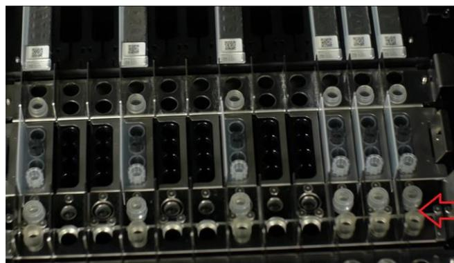
Figure 5-63: Example of Sonication Tube (bottom) and Cap (top) placement on the instrument
