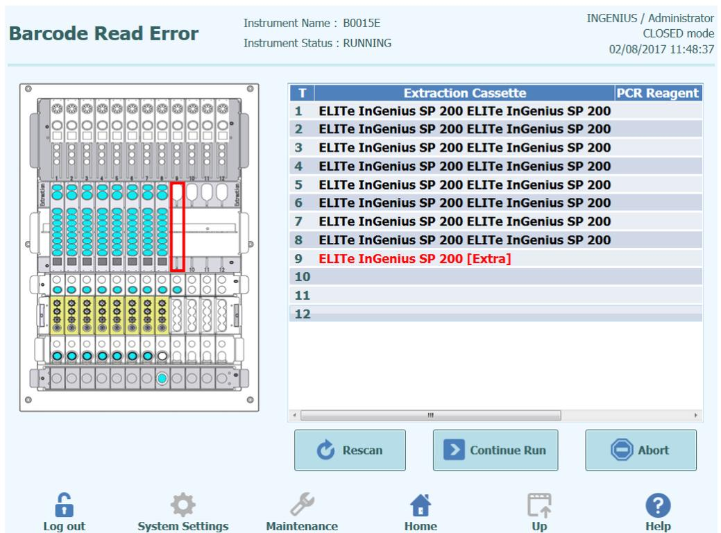
Figure 7-1: Barcode read error screen
