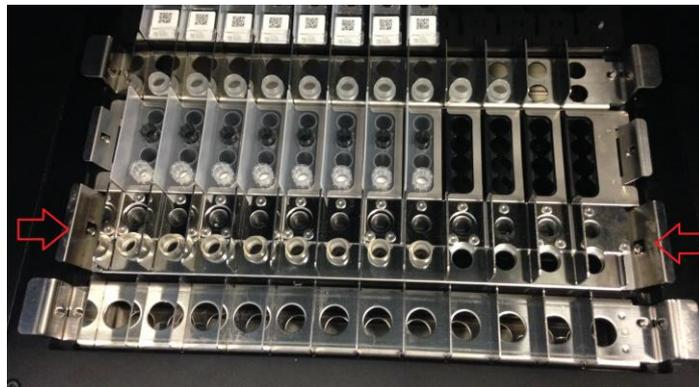
Figure 5-61: Removing Sonication Rack
