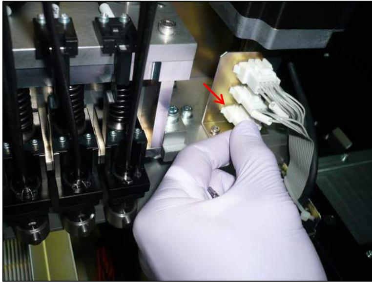
3.7.16.5 Remove the four cross slot screws (two on either end) that hold on the electrical connection brackets (Figure 229 & Figure 230)
