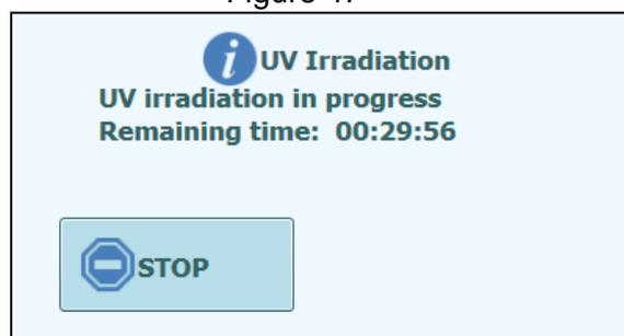
After the UV sterilization has completed, the door lock is unlocked and the system software is shutdown automatically. Once the system has completed its shutdown, you should turn off the power switch at the side of the instrument.
