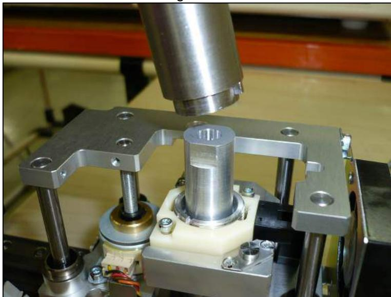
3.9.3.3 Install the ultrasonic oscillator onto the replacement UX axis using the special tool and use care not to overtighten
