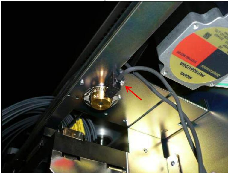
3.8.3.5 Remove the two cross slot screws that secure the org sensor(Figure 248)
