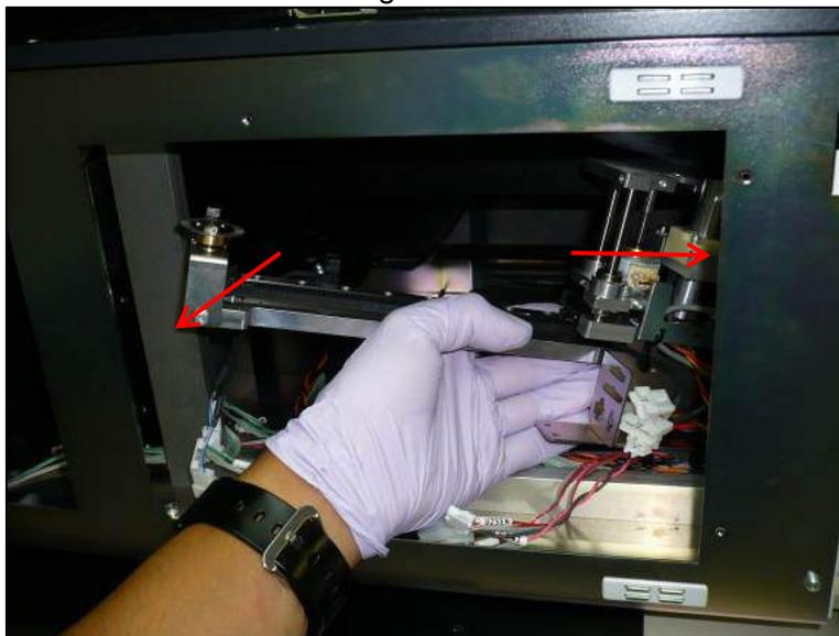
3.9.1.11 Remove the two cross slot screws from the bottom side of the module that secure the cable support (Figure 284)
