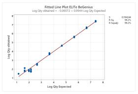
The Lower Limit of Quantification (LLoQ) was set at the LoD concentration that gives quantitative results precise (Standard Deviation = 0.3762 Log IU / mL) and accurate (Bias = 0.3583 Log IU / mL) within  $\pm 0.5 \text{ Log IU} / \text{mL}$ : 26 IU / mL.
