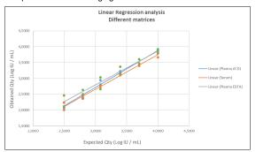
The linearity of the assay was confirmed for Plasma collected in ACD and Serum giving an R2 respectively of 0.9838 and 0.9870 and the quantitative results within  $\pm 0.5$  Log IU / mL.
