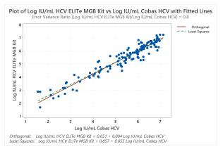
In this test, the Deming regression analysis generated a slope equal to 0.894 (95% IC: 0.846 - 0.941), and an intercept equal to 0.651 (95% CI: 0.391 - 0.911). The linear regression analysis generated an R2 of 0.916.
