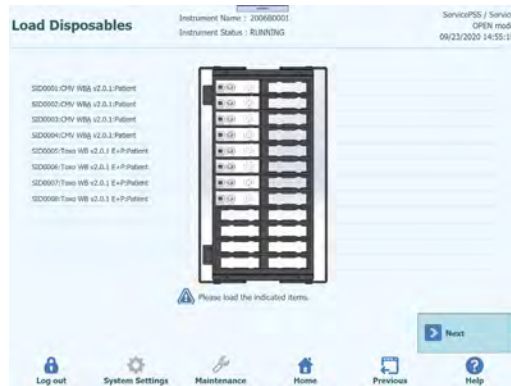
Figure 5-183: Installation of PCR cassette required for the second extraction
