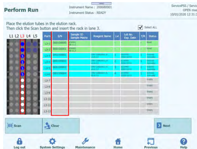
Figure 5-115: Insertion of serial number for the Calibrator reagent Tube
