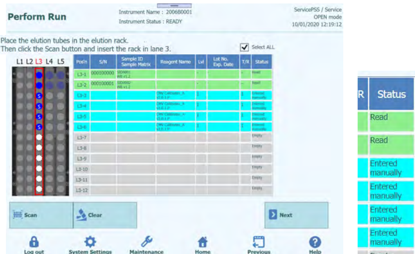
Figure 5-111: Selection of Calibrator reagent from the "Reagent Name" column
