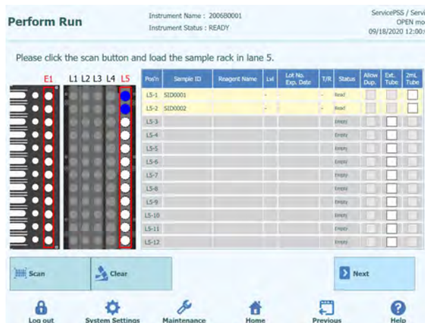
Figure 5-36: Rack barcode scan results
