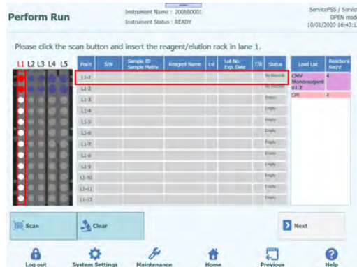
Figure 5-141: Selection of the position of the Cooler Unit where the Reagent is placed
