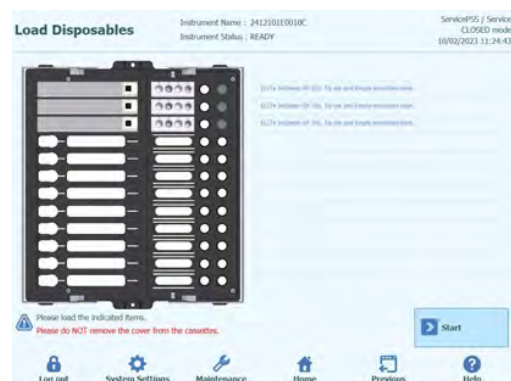
Figure 5-184: Installation of Extraction cassettes, Tip-sets and Extraction Tubes required for the second extraction
