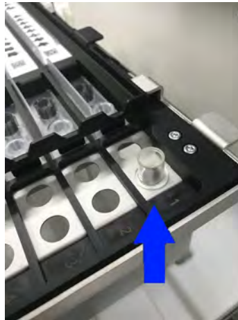
Figure 5-48: Installation of Extraction tube in the Extraction Rack
