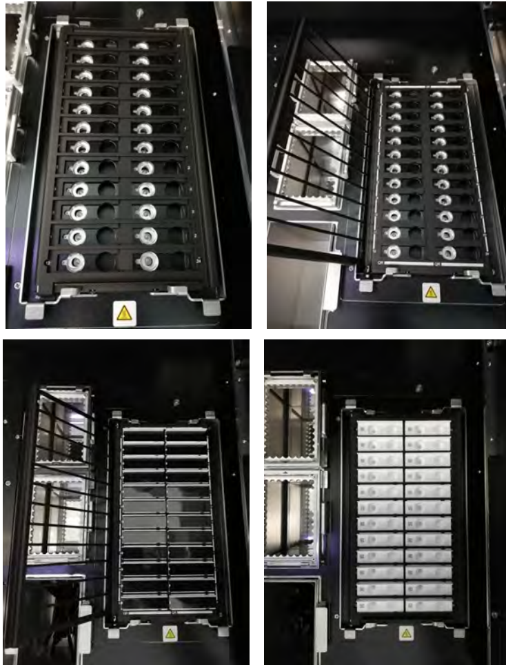
Figure 5-177: Installation of PCR cassettes on the PCR Rack of the instrument
