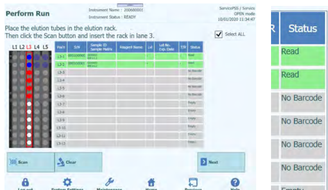
Figure 5-110: "No Barcode" status when no label is attached to the Calibration Tube
