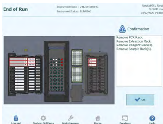
Figure 5-211: End of Run screen with instructions on unloading, storing or discarding the samples, materials and reagents
