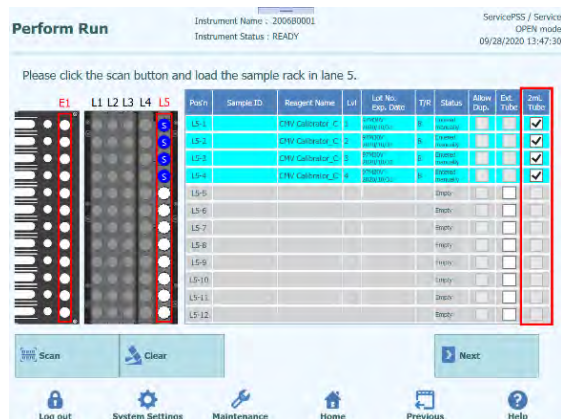
Figure 5-156: 2 mL tube check in case of 2 mL Calibrator tube
