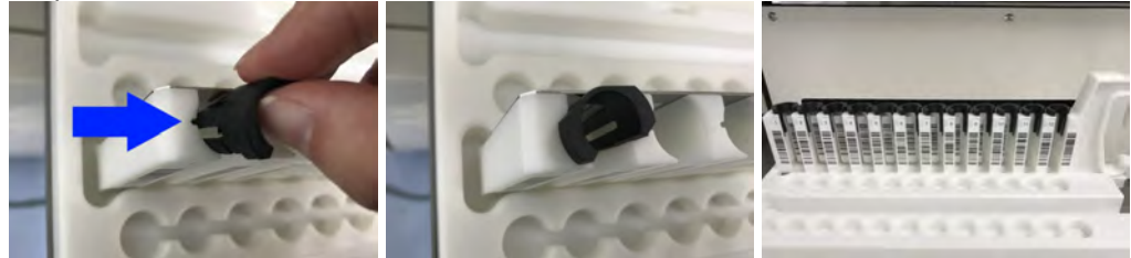
Figure 4-5: Insertion of sample rack adapters in the ELITE BeGenius rack.
