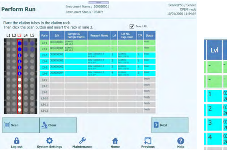
Figure 5-107: Selection of levels for the Calibration Tube
