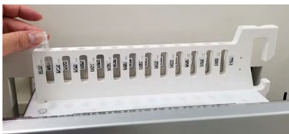
Figure 5-135: Insertion of Reagent Tube in the Rack
