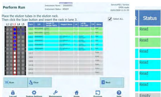
Figure 5-106: Successfully read barcoded Calibrator Tube
