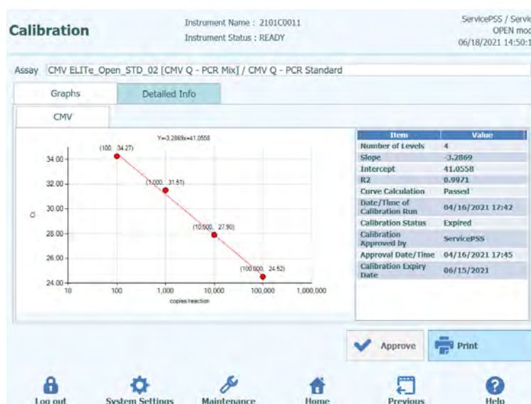
Figure 5-15: Calibration Curve - Graph screen.
