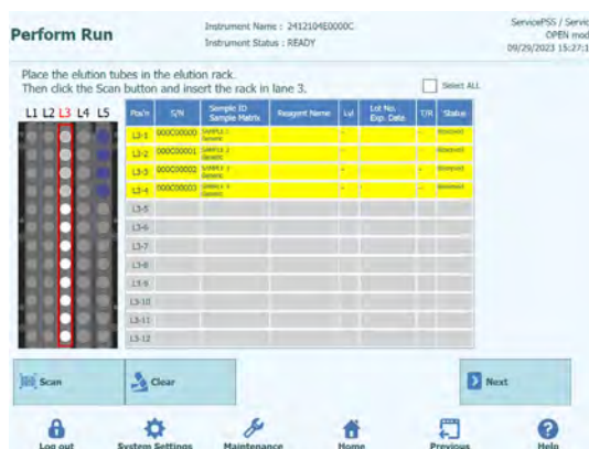
Figure 5-98: L3 Elution Rack barcode scan activation
