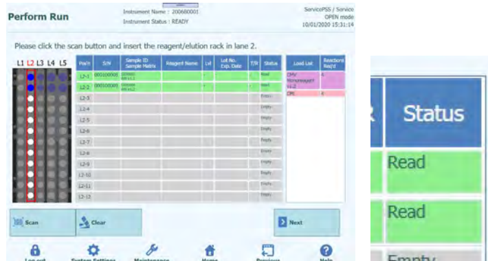
Figure 5-130: "Read" status for successfully read barcoded Eluate Tube
