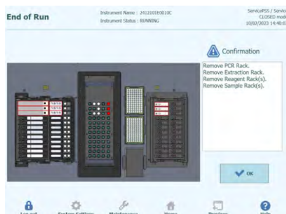
Figure 5-211: End of Run screen with instructions on unloading, storing or discarding the samples, materials and reagents
