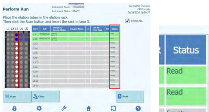
Figure 5-90: Successfully read Eluate Tube barcode
