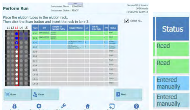
Figure 5-122: Selection of Control reagent from the "Reagent Name" column
