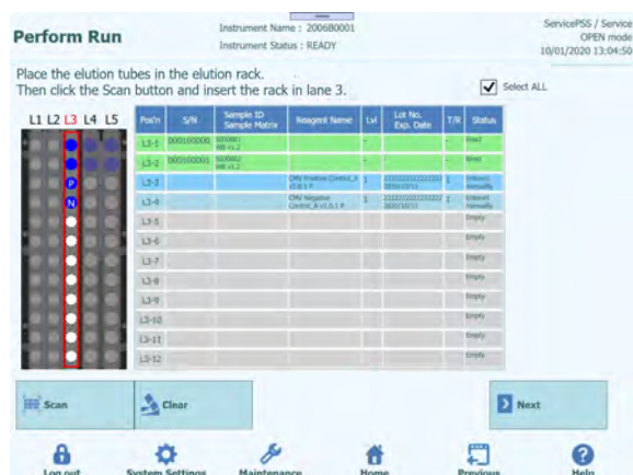
Figure 5-123: Insertion of Lot Number and Expiry Date for the Control reagent
