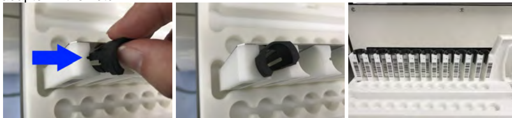
Figure 4-5: Insertion of sample rack adapters in the ELITE BeGenius rack.
