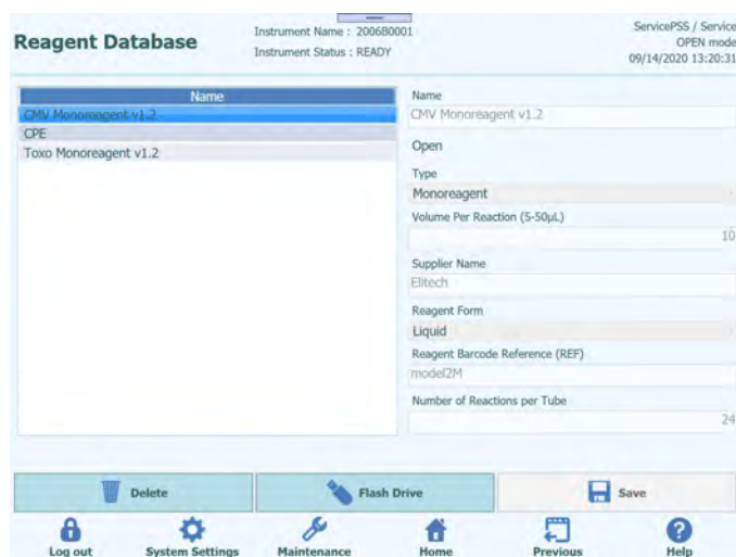
Figure 6-41: Selection of a reagent from the "Name" list on Reagent Database screen
