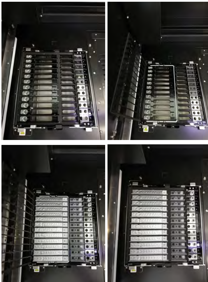
Figure 5-179: Installation of Extraction cassettes, Tip-sets and empty Extraction Tubes on the Extraction Rack of the instrument
