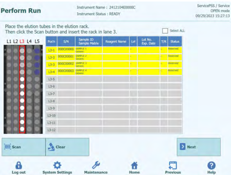
Figure 5-95: "Reserved" status for Elution tube without barcode
