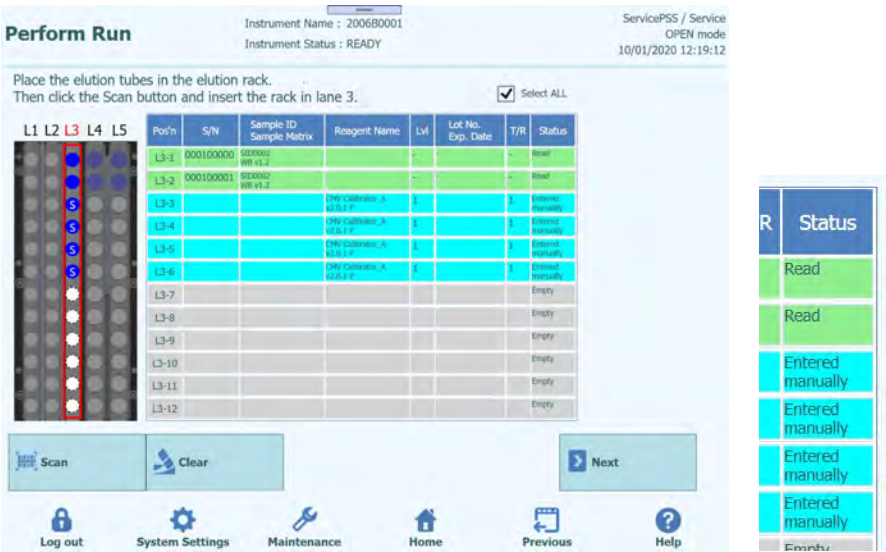
Figure 5-111: Selection of Calibrator reagent from the “Reagent Name” column
