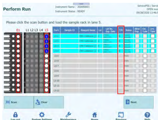
Figure 5-154: Selection of reaction number of the Calibrator tube
