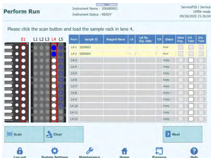
Figure 5-72: Successfully scanned Sample Tubes
