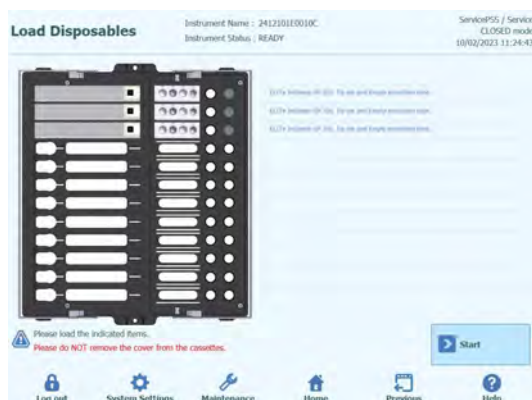
Figure 5-178: Installation of Extraction cassettes, Tip-sets and Extraction Tubes required for the run
