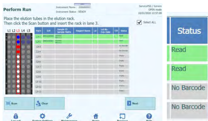
Figure 5-121: "No Barcode" status when no label is attached to the Control Tube
