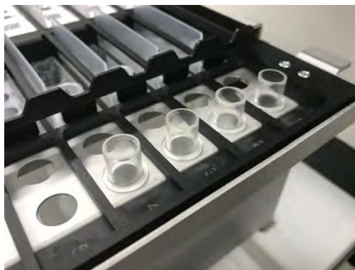
Figure 5-162: Insertion of Extraction tubes in the Extraction Rack
