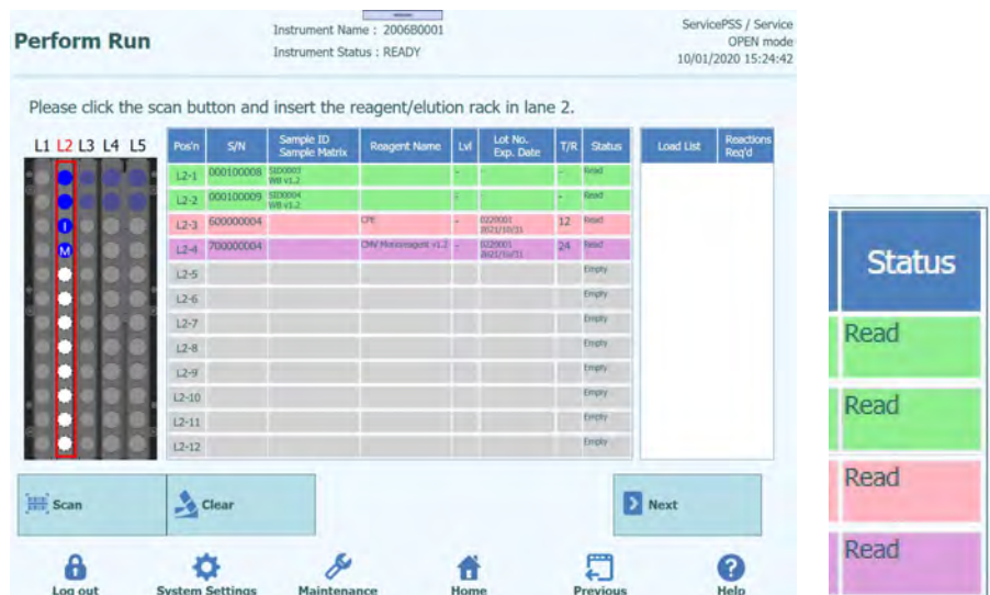
Figure 5-132: "Read" status for successfully read barcoded Reagent tubes
