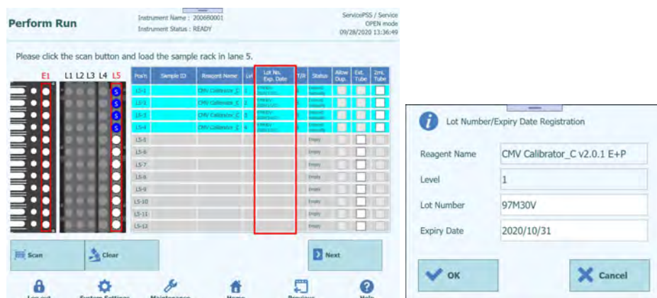
Figure 5-152: Insertion of Lot Number and Expiry Date of the Calibrator
