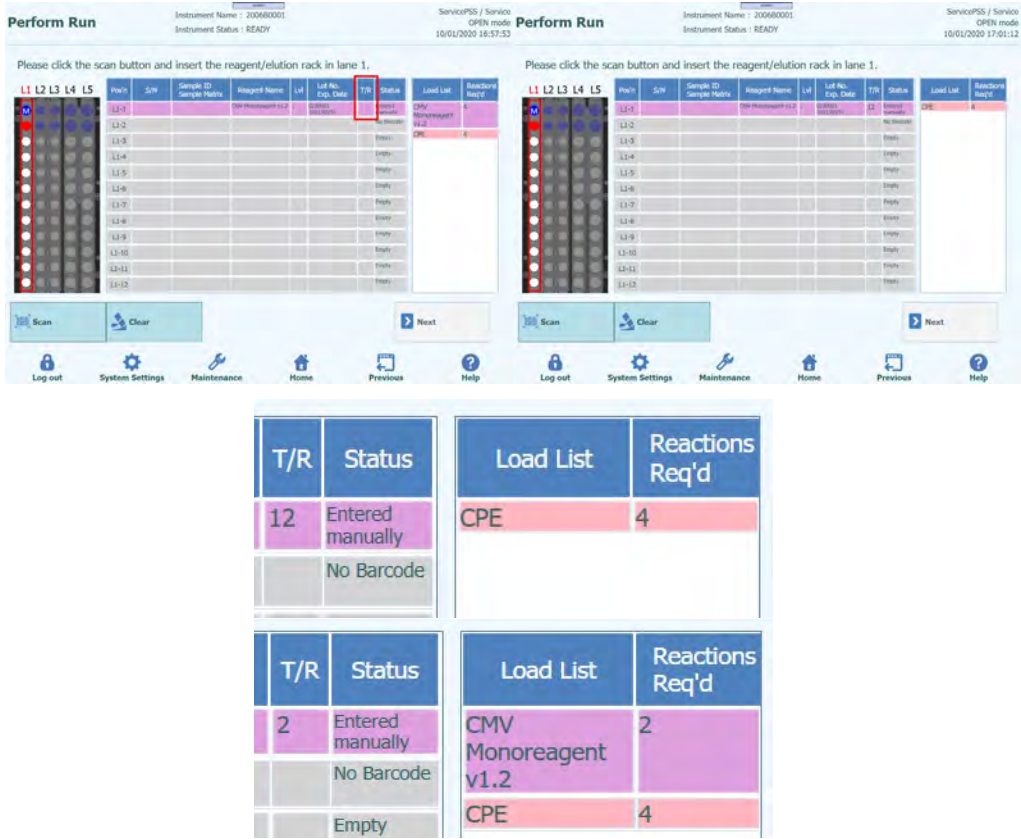
Figure 5-144: Insertion of number of reactions for the Reagent Tubes
