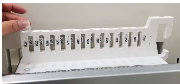
Figure 5-128: Insertion of empty Eluate Tube in the Rack
