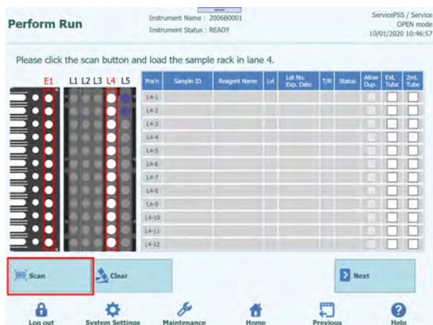
Figure 5-71: L4 Sample Rack barcode scan activation
