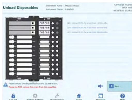
Figure 5-182: Disposing Extraction cassettes, Tip-sets and Extraction Tubes used in the first extraction
