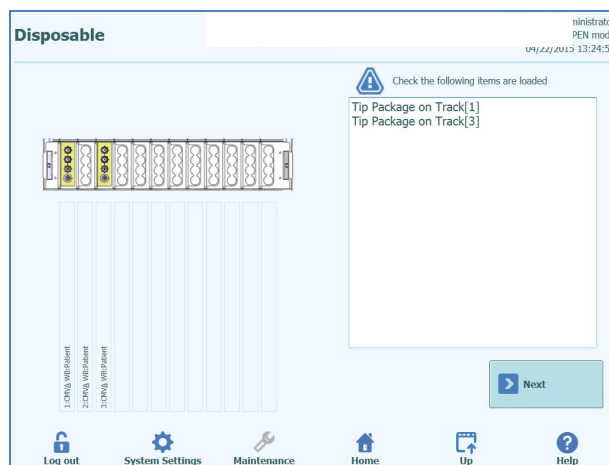
Figure 10: The “Disposable” screen is used to confirm loading tips racks
