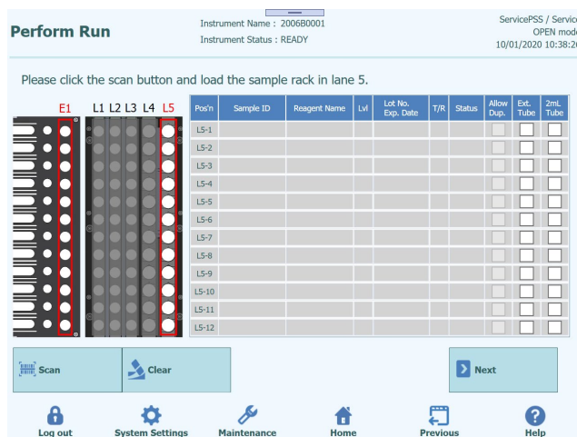
Figure 21 : Run Setup Rack Insertion
