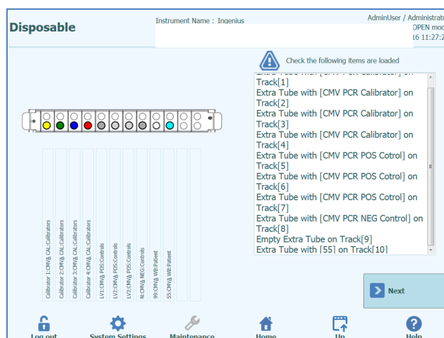
Figure 9: The “Disposable” screen is used to confirm loading of Extra Tube Rack with elution tube
