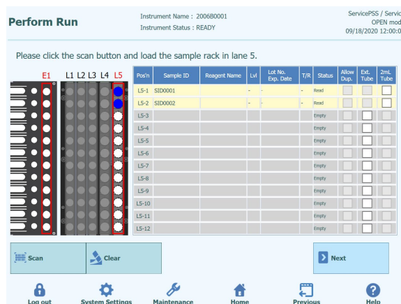
Figure 23 : Rack barcode scan results
